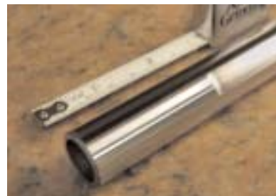
This detail of a 44"-long slide rail shows a 0.300"-wide ground area that stops 2" from the end of the tube.
