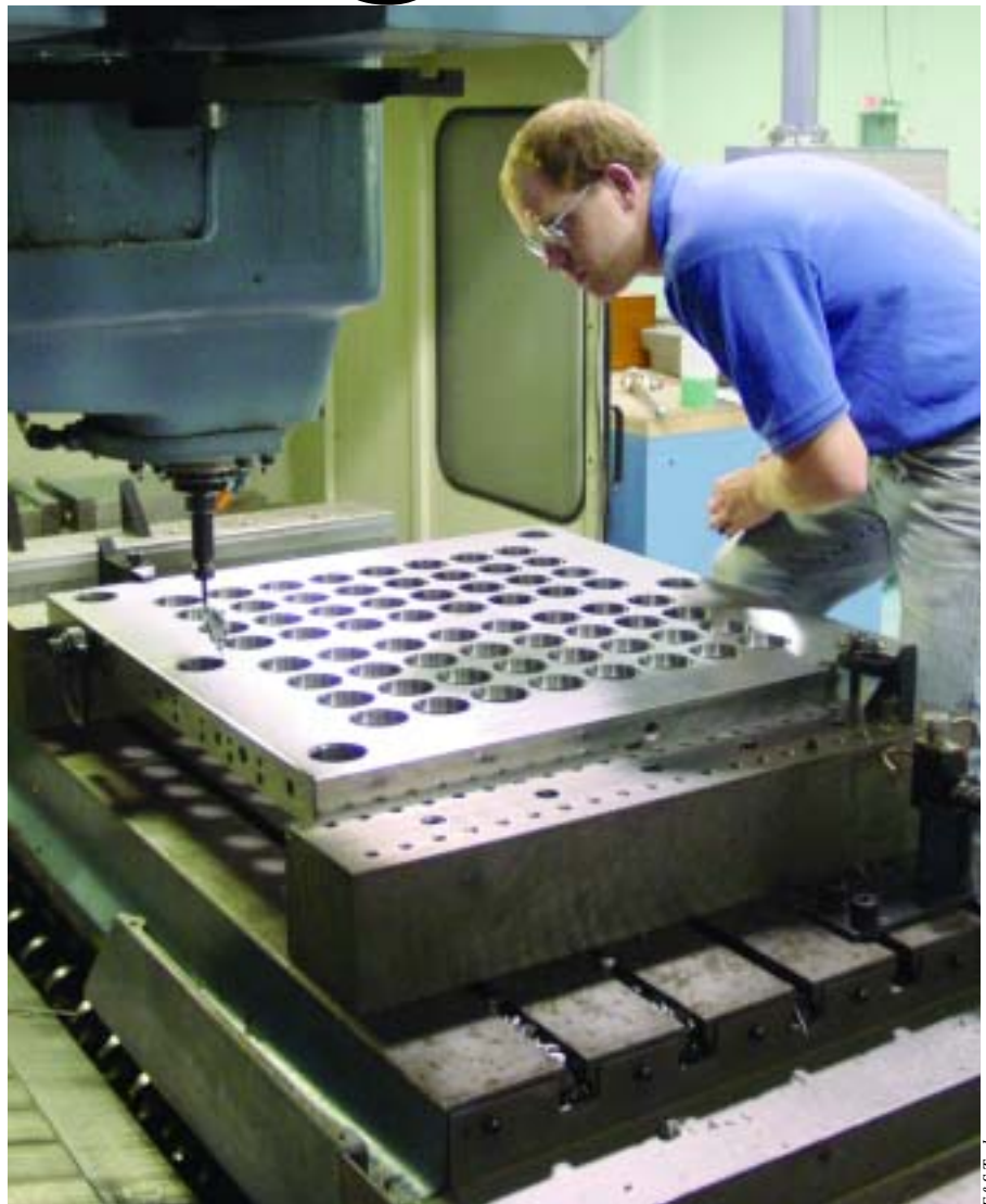
A machinist gages a rough-drilled, high-cavitation mold plate at F&S Tool.
