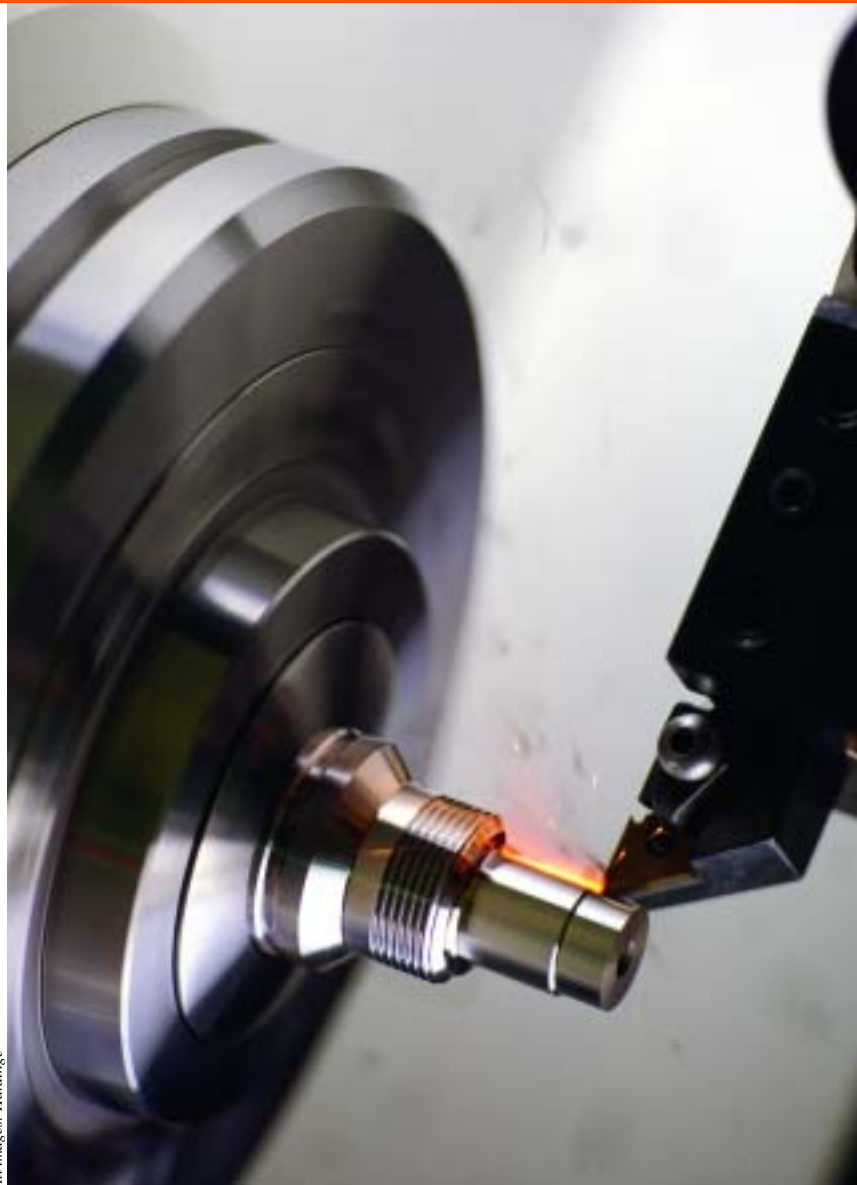
Hard turning a shaft.
