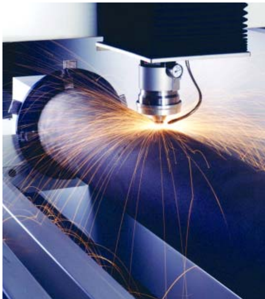
Figure 1: Tubular and structural shapes that have historically been machined can now be cut on rotary-chuck lasers with 3-D cutting torches.
