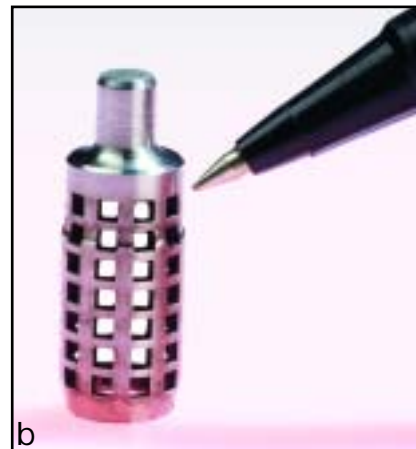
Figure 4: Most of the features on these parts were cut with a rotary laser, one (a) from a 3/8"-thick, 10"-dia. 4140 carbon steel tube and the other (b) from 2"x2' cylindrical bar stock of the same carbon steel. Unlike previously milled versions, these parts can be made on one machine. Switching from one part to the other can be accomplished in less than 5 minutes.
