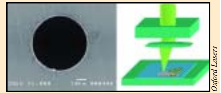
Trepanning holes with a laser provides greater machining flexibility than percussion drilling.
