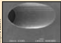
The entrance of an angled hole laser-drilled in stainless steel. Because of the shallow angle, such a hole couldn't be produced by conventional cutting methods.
