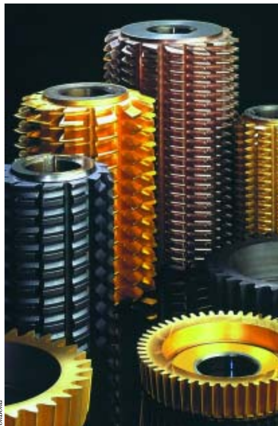
HSS hobs, shaper cutters and a broach, all with TiN coating.
