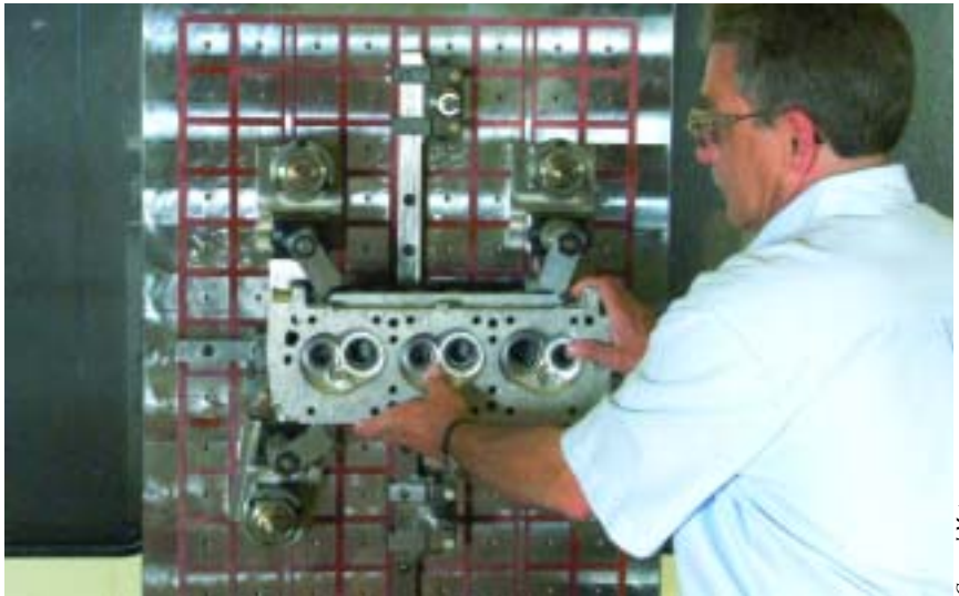
Phil Bojda, senior research engineer with GM R&D, demonstrates GM's new agile machining fixture, which incorporates modular, self-contained elements.
