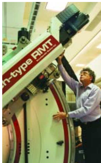
This prototype RMT, designed by the ERC/RMS and built by Masco Machine, offers enhanced functionality by fitting a milling/drilling spindle on an adjustable arch-shaped mount.
