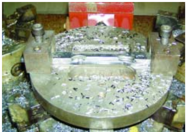
A rigid setup is critical when cutting exotics, such as titanium.
