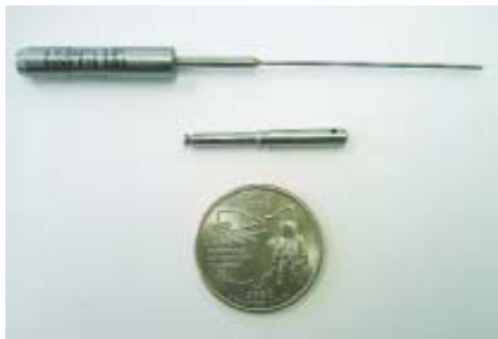
A 0.032"-dia. x 1.25"-deep gundrill was applied to make this dental drill.
