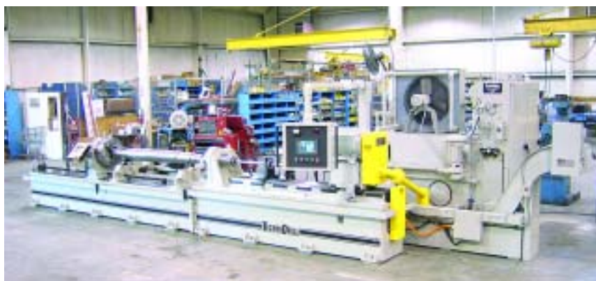
A 2.00"-dia. x 50"-stroke BTA machine was used to drill alternator shafts for power generators.
