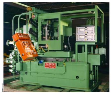
The older size-control system shown here incorporates four pneumatic controllers—one each for the two tool positioners and one each for the two pneumatic gage heads. Newer SCS controllers, such as Samsomatic's Model SC3, save floor space. A single SC3 can perform the work formerly done by four pneumatic controllers.
