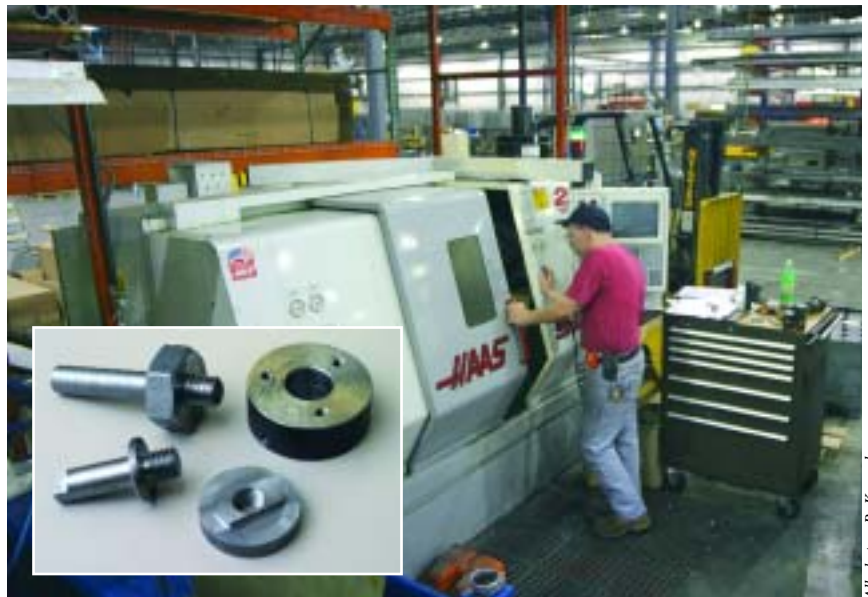
Datum Filing Systems uses a Haas SL-20 CNC lathe with live tooling and a C-axis drive to machine connector “donuts” and chain-tensioner components (inset).
