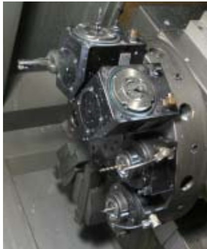
The lathe's 10-tool turret (above) is fitted with drills for axial (upper right) and radial drilling of steel wheels for filing cabinets.
