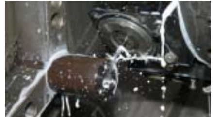
The lathe's 10-tool turret (above) is fitted with drills for axial (upper right) and radial drilling of steel wheels for filing cabinets.
