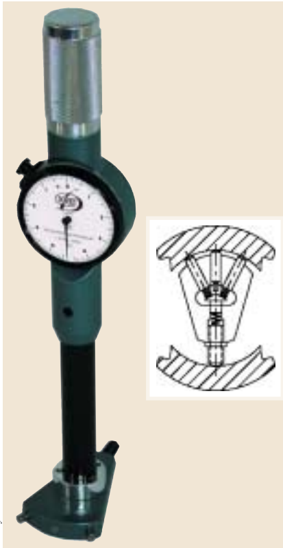
A tipping bore gage with two measuring contacts and two centralizing plungers. Inset: Diagram of the tipping bore head.
