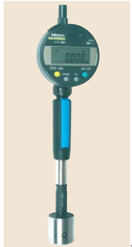
Indicating plug gages are similar to GO/NO-GO gages but they have contacts that provide a reading.
