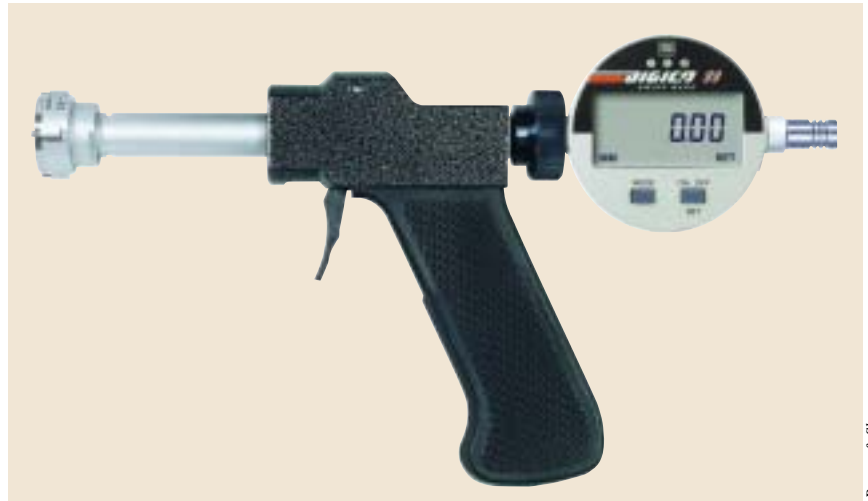
A 3-point gage can detect lobing in bores.
