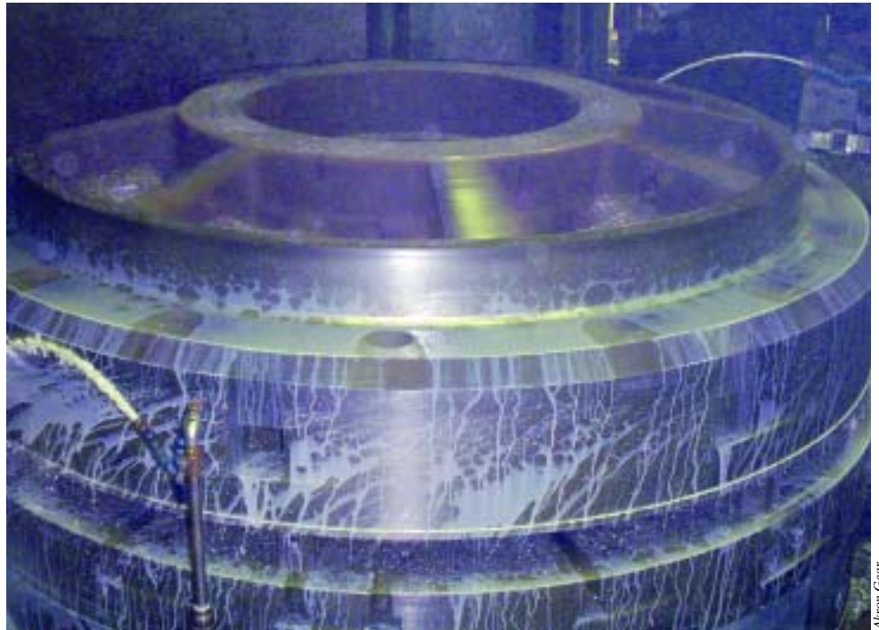
It took 30 hours to OD- and ID-turn and counterbore this 109"-dia., 24"-high, 18,000-lb. casting on a Bullard Dynatrol VTL at Akron Gear & Engineering.
