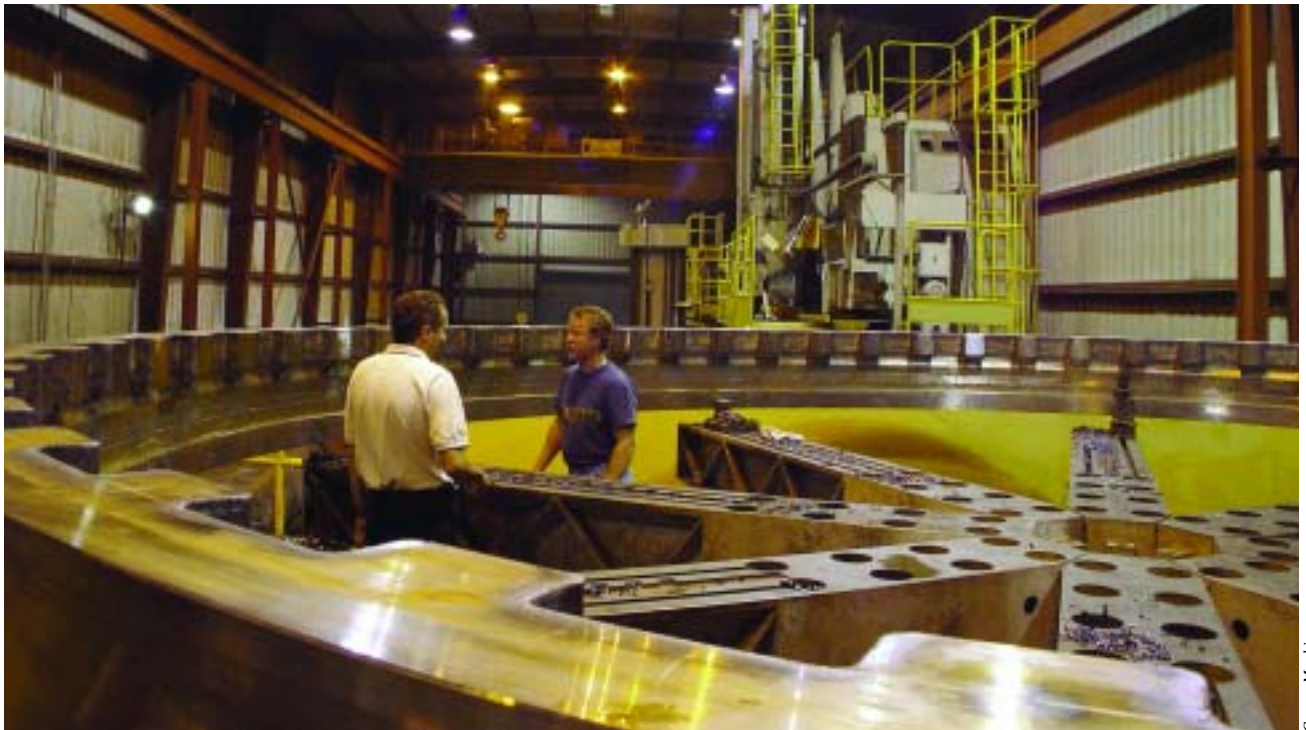
Camco Machine turned this 24'-dia. steel ring, part of a set for an autoclave door, on one of its Osaka Machine Tool VTLs.
