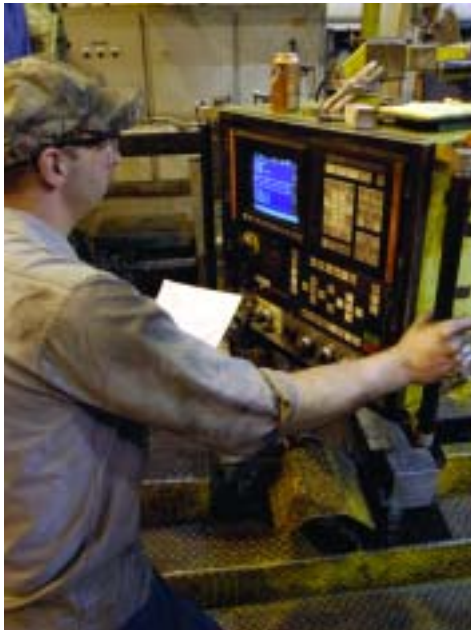
Operator John Taydus at the NUM CNC that was retrofitted to the Farrell lathe at Grand Valley Manufacturing.
