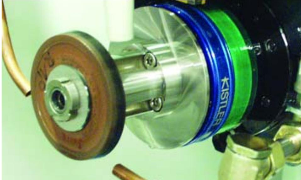
The use of superabrasive wheels with phenolic-resin bonds is growing among manufacturers of carbide cutting tools.
