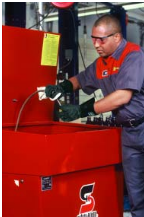
Parts cleaners with automated solvent recycling minimize waste. Shown is Safety-Kleen's Model 250.
