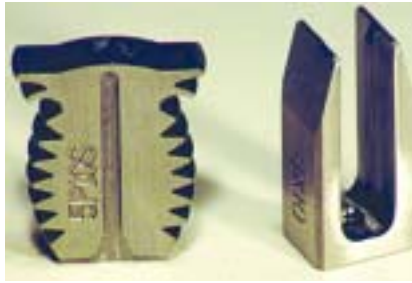
These spinal implant devices are made of Ti-6Al-4V-ELI and machined complete on a 12-axis Tornos Deco machine.
