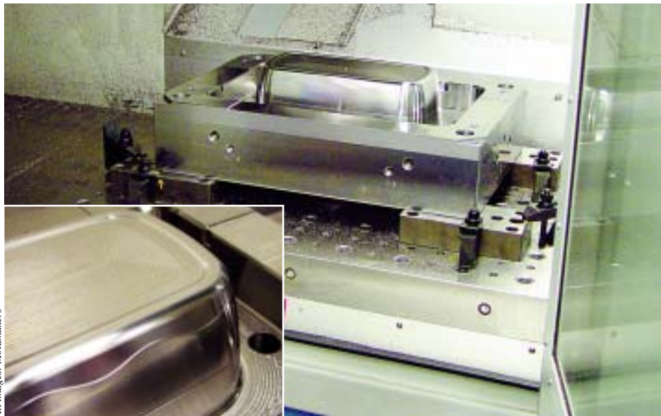
The core of a mold for a food storage container is machined out of P-20 on a Roeders 800.
