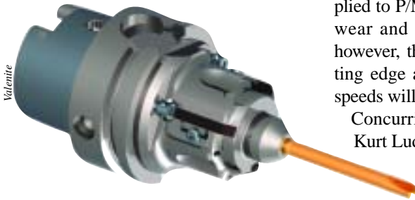
Valenite developed this solid-carbide, 2-flute reamer to machine P/M valve seats. The tool features a PCBN blade.
