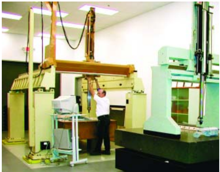
Coordinate measuring machines are used for inspecting finished parts.
