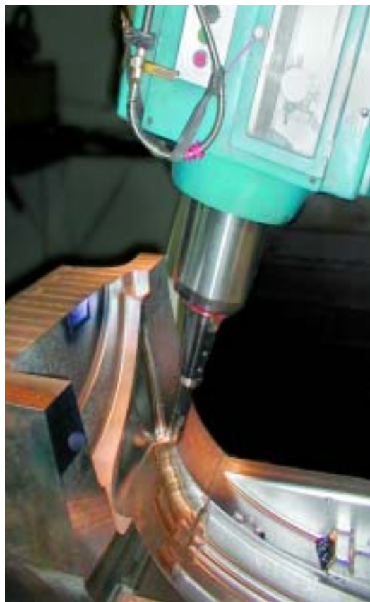
Five-axis machining of an automotive bumper mold is accomplished with toolpaths created in Delcam's PowerMILL CAM software.
