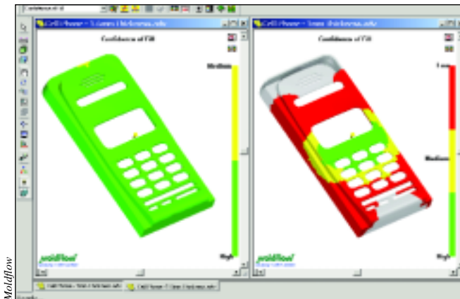
Color-coded simulations enable users of Part Adviser software to determine the manufacturability of plastic part designs early in the design process.
