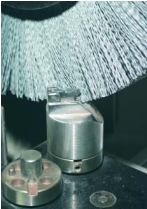
Dense silicon-carbide filament brushes hone a cutting tool, which is precisely directed by a CNC.
