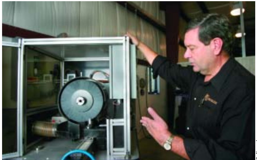
Conicity Technologies' Bill Shaffer monitors a brush honing machine he developed to create uniform or variable edge preparations.
