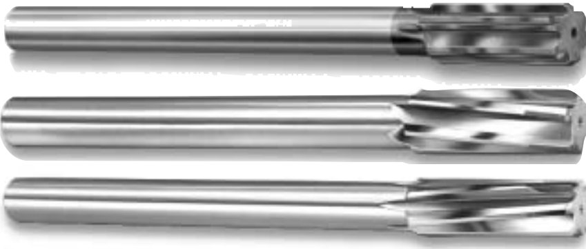
Figure 1: A straight-flute reamer is best suited for finishing shallow holes in short-chipping materials (top). Center: A reamer with right-hand spiral flutes is effective for blind-holes in long-chipping materials. Bottom: The action of the left-hand spiral flutes tend to push the reamer back into the spindle, which benefits overall rigidity and provides for accurate control of the hole diameter.
