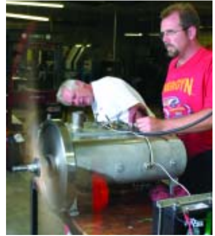
Hesler and a staff member test-run the engine with a dummy wooden propeller.
