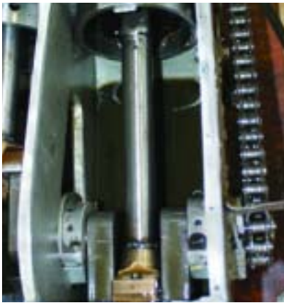
Closeup of one cylinder's connecting rod and crankshaft journal. At the top is a cylinder that was threaded and screwed into the engine block.
