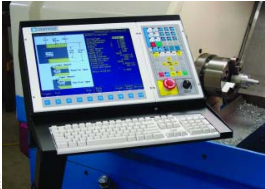
Replacing an old control with a new one, such as this Centroid T-400 CNC for lathes and turning centers, can enable an old machine with good iron to run better than new.
