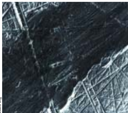
Micrographs of a coated drill showing the wear to the top-layer MoS 2 coating after 50 rotations (top) and 400 rotations.
