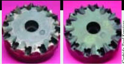
A 10"-dia. facemill before (left) and after repair.
