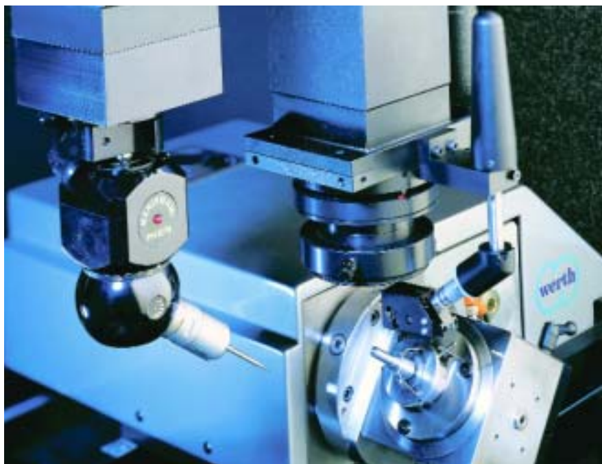
A Werth America system inspects a diesel fuel-injector nozzle using touch, laser and video probes. Mounted below the camera is the company's fiber-optic probe, one of the new probe styles recently introduced to industry.
