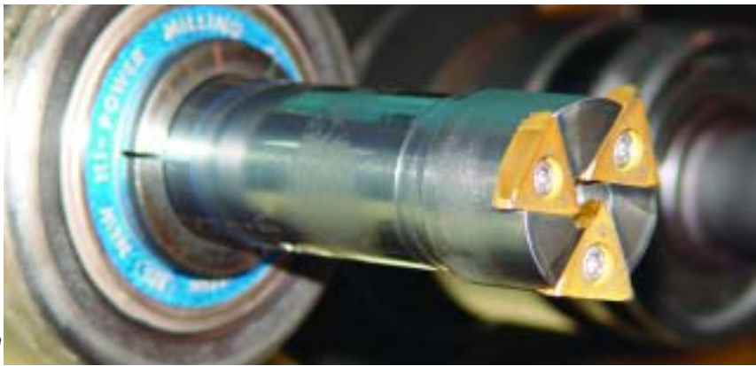
A special undercut tool with triangle-shaped inserts from McQuade Industries.
