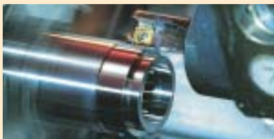
A single EcoCut tool drills, bores, chamfers, faces and turns.
