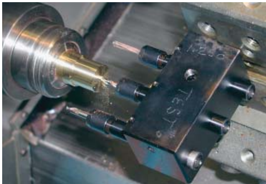
Foxwood Machine developed the Turretgang to lower turret-indexing time. Soon after, the shop began selling the multitool holders to other companies.
