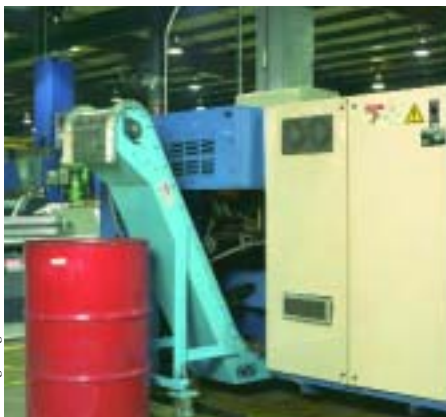
Beltless magnetic conveyors allow ferrous chips to travel along a steep incline and handle sharp, abrasive parts and scrap that can damage conveyors with belts.
