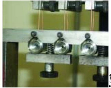
Abet Industries designs and builds its own EDM holemaking machines and power supplies. Here, 20 holes are being EDMed simultaneously.
