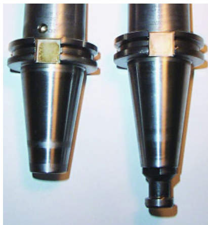
The toolholder on the left shows wear lines, which are a result of an overtightened retention knob.
