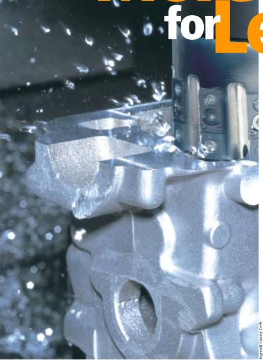
Today's tougher-to-machine aluminum alloys require advanced PCD materials and tools.
