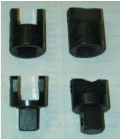
The U-joints Abrasive-Form tested were made of 4140 steel.
