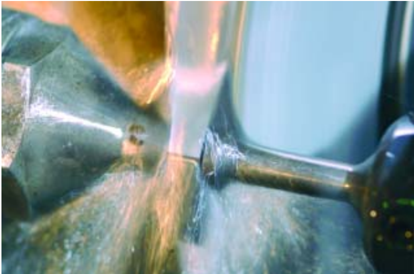
Agathon's EcoDress process electrochemically dresses wheels, reportedly reducing cycle time by up to two-thirds.
