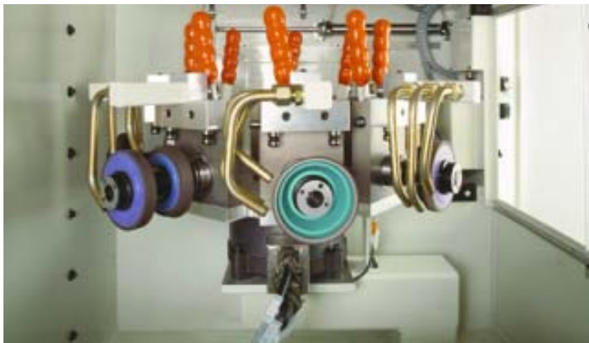
The UW ID grinder swaps out wheels and nozzles automatically.
