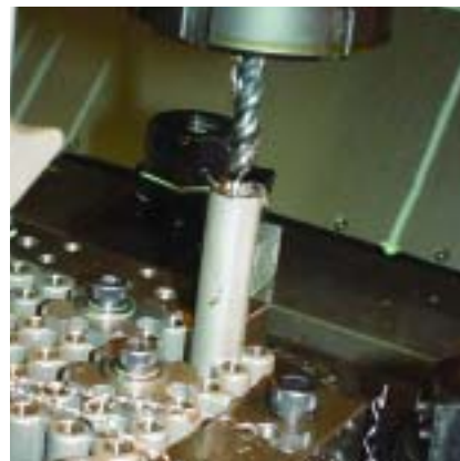
Diamond Tool & Die uses Prototyp's Triple-S tap to thread holes 3 diameters deep in 304 stainless steel.
