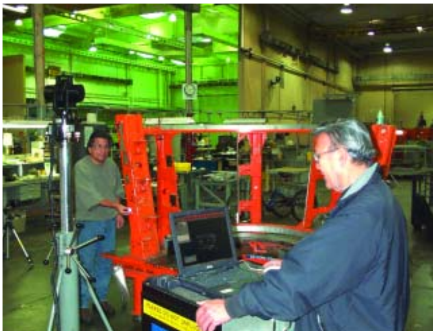
Reworking an assembly jig to engineering specifications.
