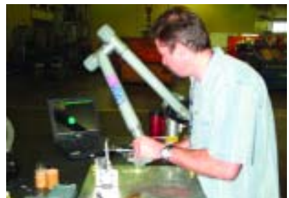
Locating the details on a weld jig using a portable measurement arm.
