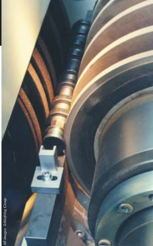
Figure 1: Grinding of camshaft bearing journals using high-speed centerless grinding and CBN grinding wheels.
