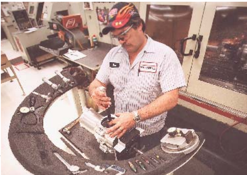
Next to the machining center Don Anthony runs is an inspection bench he created to help speed and optimize the inspection of parts produced at his workstation.
