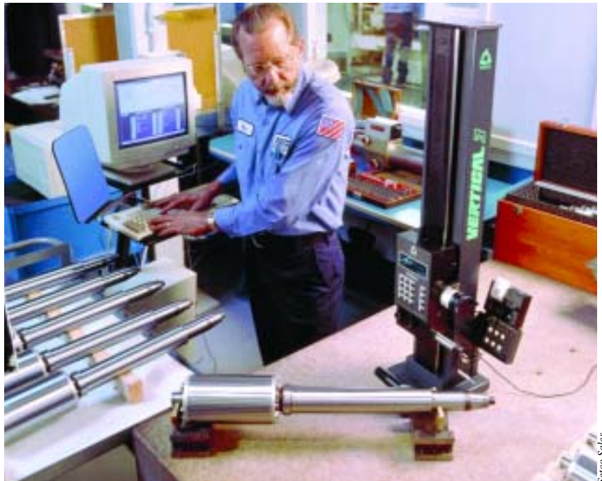
Critical part-print tolerances of spindle surfaces are being measured to ensure vibration-free operation.
