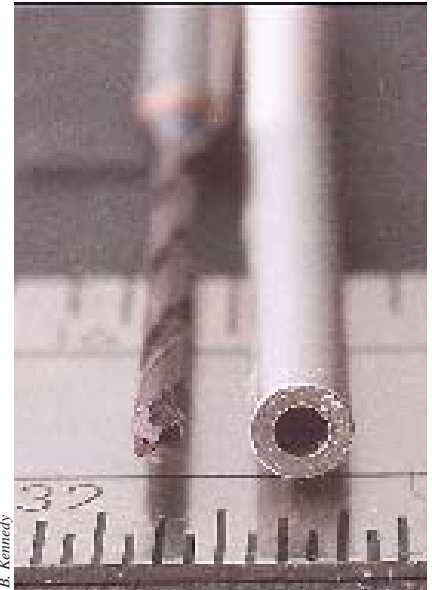
A solid-carbide, 0.055"-dia., through-coolant drill from Mitsubishi (left) is used to drill a 0.0525" hole in a 302 stainless steel medical component (right). Units on the ruler are \frac{1}{32} ".
