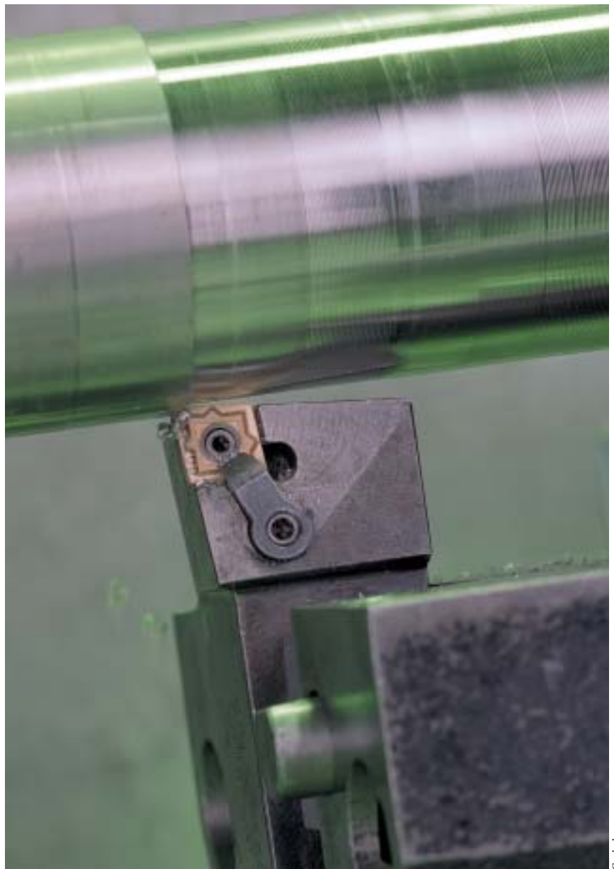
Turning titanium has become progressively easier with the right tools, such as, in this case, Carboloy's CP200 PVD-coated carbide turning grade.
