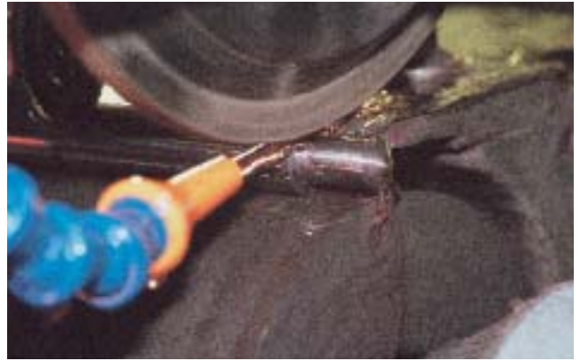
Qualified machinist Brandon Beech (left) works with Tru Tech software in a grinding cell at AGS to carry out such operations as centerless grinding of carbide tool blanks (right). Beech said the software enables him to grind complex contours while tending to two other machines.
