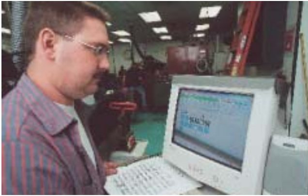
Qualified machinist Brandon Beech (left) works with Tru Tech software in a grinding cell at AGS to carry out such operations as centerless grinding of carbide tool blanks (right). Beech said the software enables him to grind complex contours while tending to two other machines.
