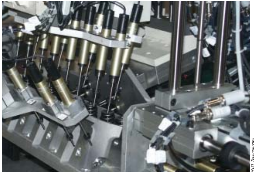
At General Motors' engine plant in Romulus, Mich., an eddy-current test system checks multiple tapped holes simultaneously.
