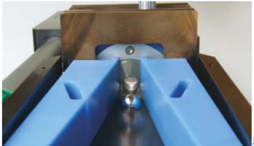
Besides tapped holes, eddy-current technology can also test ball bearings.
