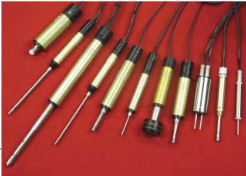
Eddy-current thread probes can be placed in a toolholder and become part of the machining process.
