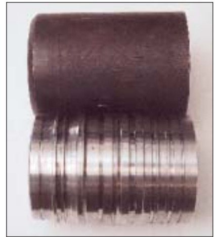
Horizontal lines are scribed into a steel forging of an intermediate hub for an automobile transmission. The depth of the scribes varies from 0.032" to 0.265".
