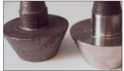
An 8625-H alloy steel, scribed stem pinion for an automobile rear axle (left) and a similar part after machining. The range of the depth of the scribing is 0.005" to 0.026".
