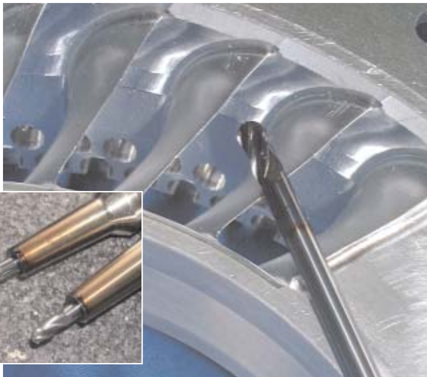
Coated 4mm, 4-flute ballnose endmills are used at Tech Development to machine complex internal contours on aerospace parts. The cutters are held in shrink-fit toolholders (inset).
