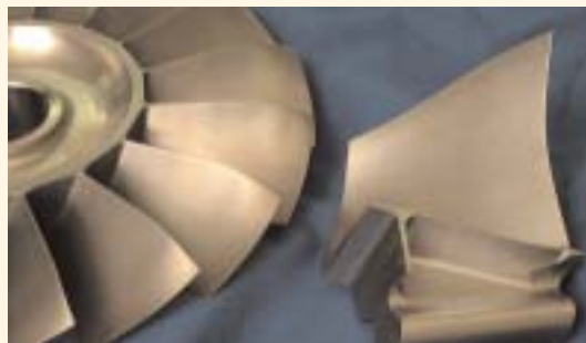
Endmilling components made of titanium alloys, such as these aerospace parts machined by Tech Development, requires tools with high helixes and rake angles to minimize friction.
