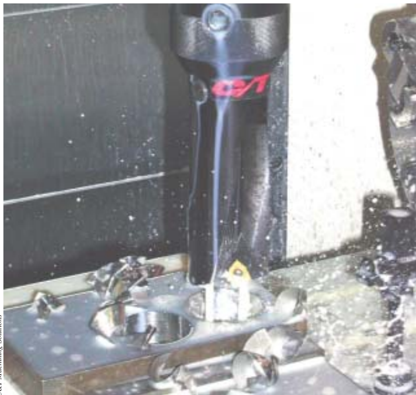
A 1.5"-dia. indexable drill with high-pressure, through-spindle coolant.
