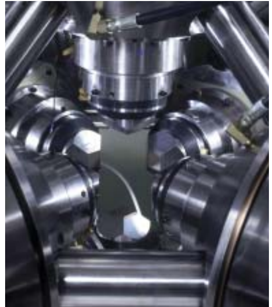
Precorp's high-temperature, high-pressure press can achieve pressures of 3 million psi and temperatures of 3,632° F.
