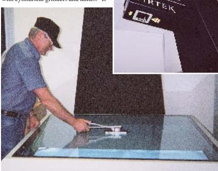
Del Rohloff, a quality assurance technician at outdoor equipment maker The Toro Co., uses a magnetic gripper to place a part onto the scanning table of a LaserQC laser inspection system from Virtek Vision International Inc. A laser projector mounted above the table (inset) casts the laser beam onto the part to capture more than 500 data points per second. Software superimposes the scanned image onto a CAD reference image, and the tolerances are color coded to reveal any variances.
