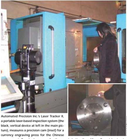
government. Required accuracy for the cam is better than 10 $\mu$ m. By not having to remove the part from the machine tool for inspection, production throughput was improved more than 200 percent.
