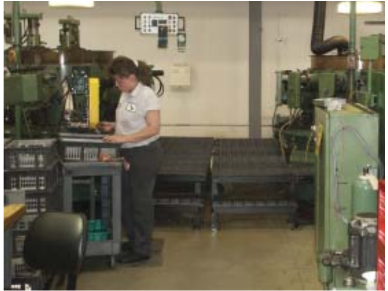
At Component Bar Products, two machines are grouped together to allow one machinist to operate both.
