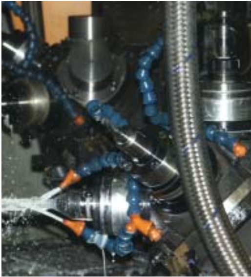
A single station in an Imasflex rotary transfer machine can have up to four spindles.
