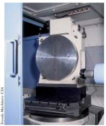
There will be no shortage of 5-axis technology on display at IMTS. For example, Toyoda Machinery USA will mill a steel drill for rock boring on its FA630 HMC. A Tsudakoma table with a C- over B-axis configuration will be used to place the part in a horizontal position—with rotary capability—over the machine's 4th axis (perpendicular to the table). This improves access to the part's raised surfaces, indentations and angles and allows complete machining in one clamping.
